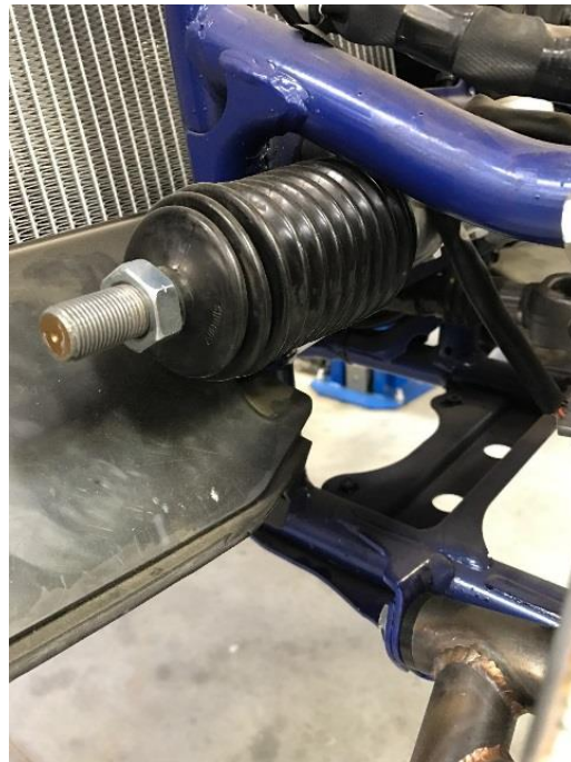
Figure 3: Steering boot installed over heim.
