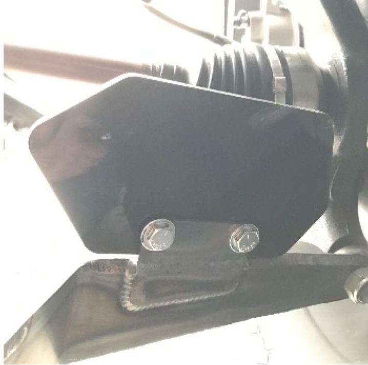
Figure 5: Rock guards installed.
