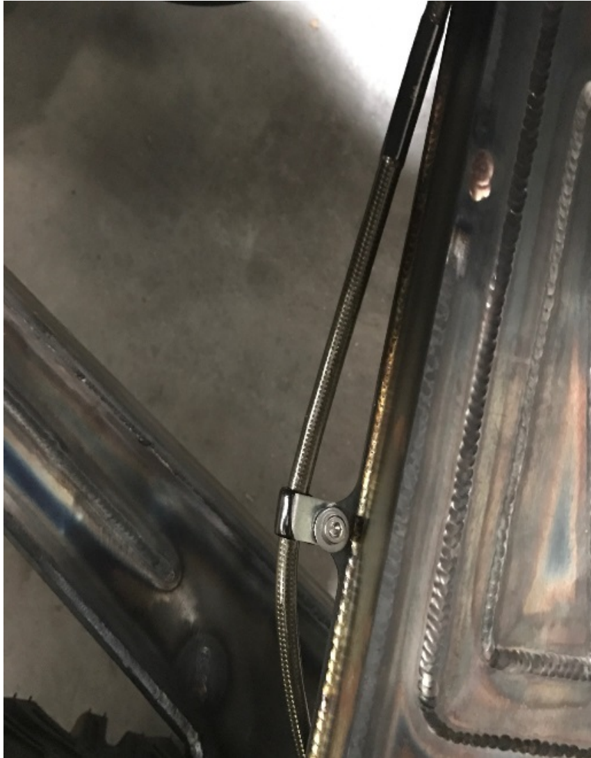
Figure 2: Route brake lines in front of the shock as shown.
