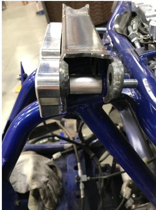
Figure 5: M10 bolts through front saddle, spacers, and through the other side.
