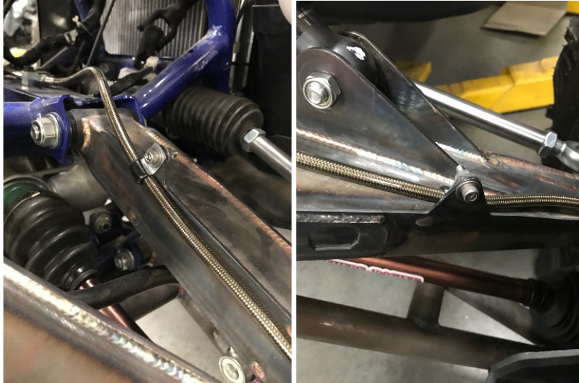
Figure 2: Route brake lines in front of the shock.
