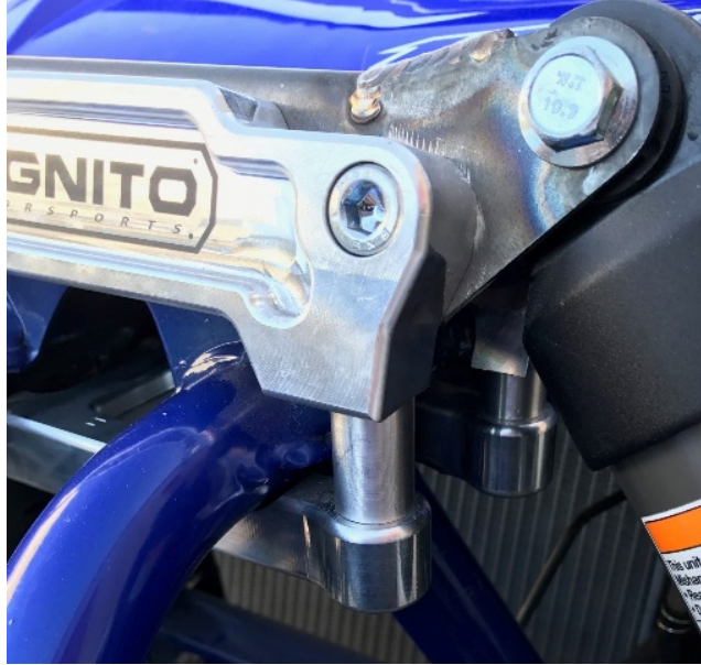
Figure 8: 4 bolts into saddles.
