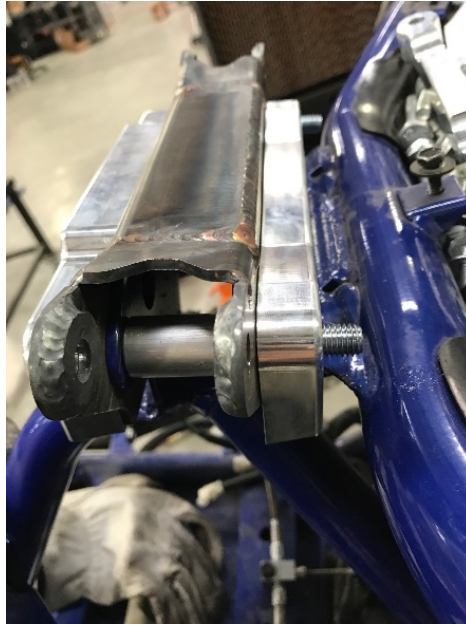
Figure 6: Back saddle in place.
