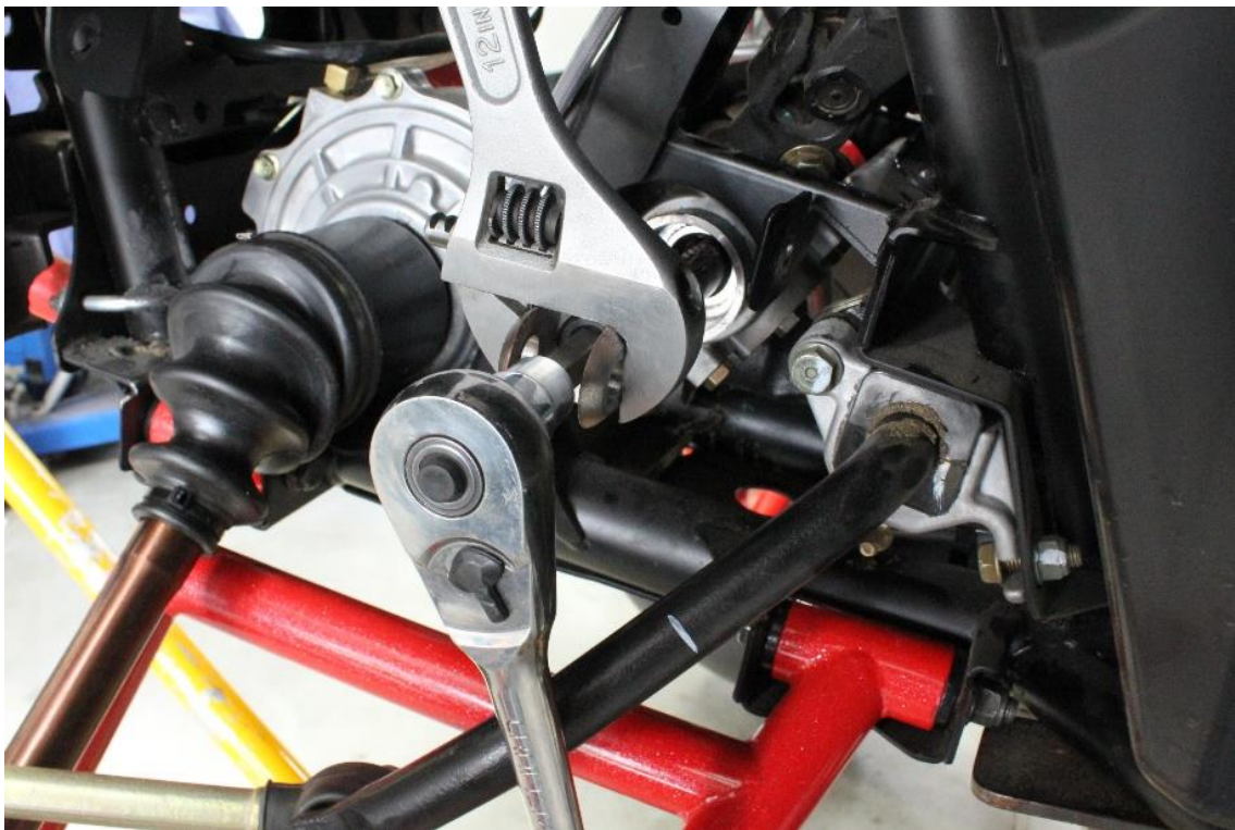
Figure 2: installing clevis to the steering rack bar
