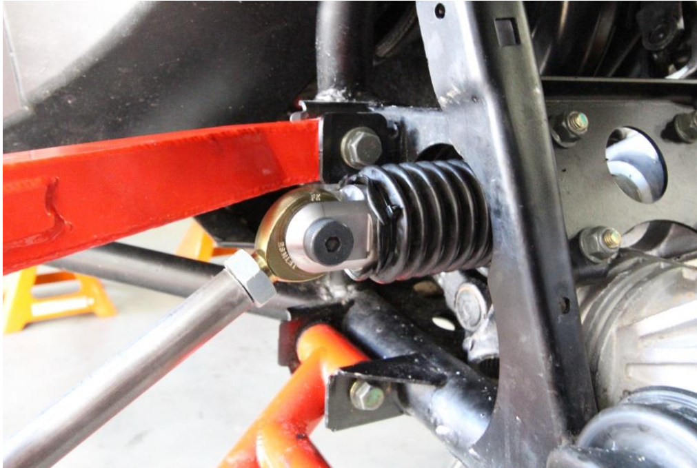
Figure 4: inner rod end attached to clevis, and dust boot tied to clevis groove.
