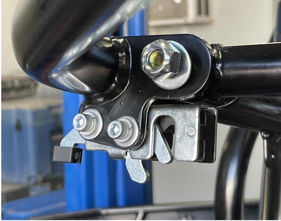
16. It is time to align the swing frame. Carefully lower the swing frame to engage the striker bars on the support bracket assemblies. Note that height of the striker mounts and the forward/rearward position of the swing frames are adjustable via slotted holes. Using these adjustment points, move the swing frame to the desired position. Follow the adjustment tips below:
