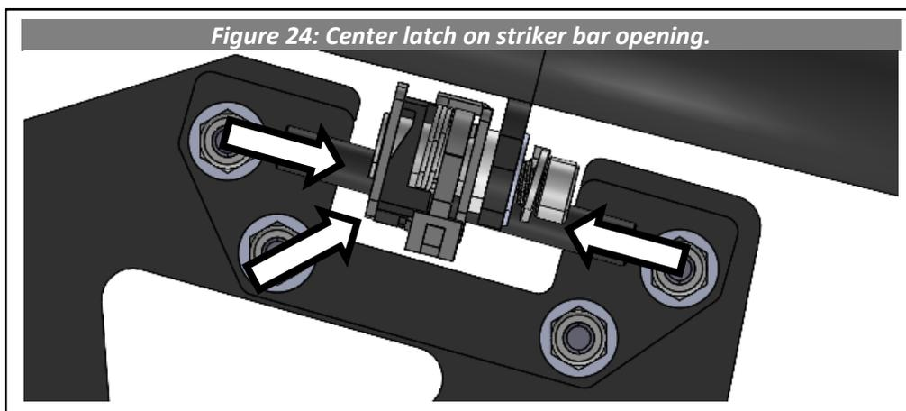
17. Confirm again that the swing frame can open and close freely and the latches are properly engaging. If so, the swing frame adjustment is complete. Beginning torquing all swing arm hardware.
