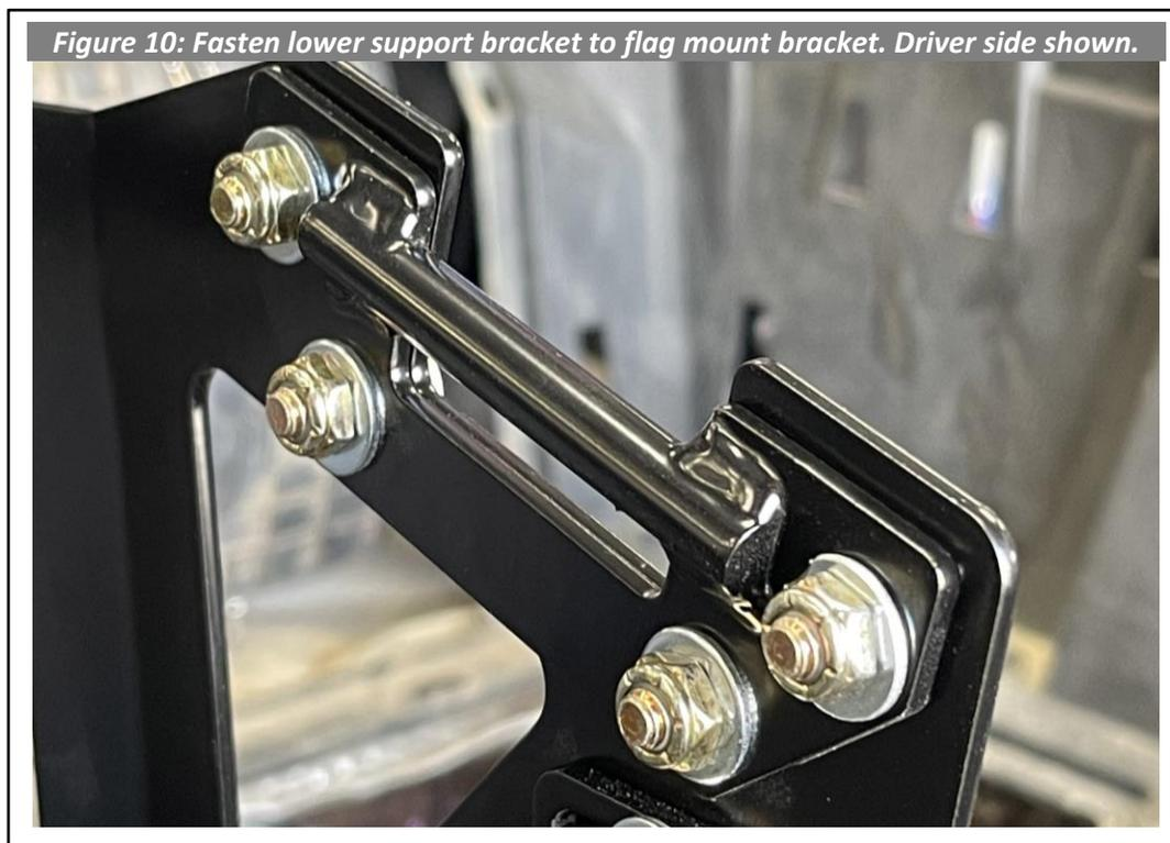
10. The spare tire lower support assembly is complete. Torque hardware to following:
