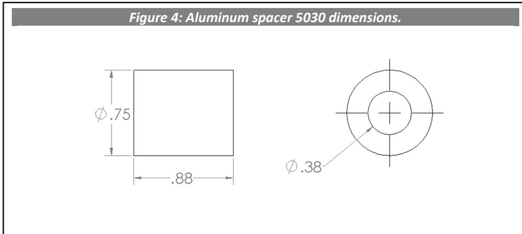
Clean any debris from bedliner pockets. Place one 5030 spacer into each pocket in the bedliner. Pass M6 bolts through 1/4" washers, foot brackets, then spacers, and thread into chassis. Orient foot bracket as shown in **Figure 5**. Long slot should be vertical. Tighten until secure but do not torque.
