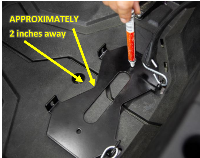
Figure 2: Positioning Mounting Base for Markings
