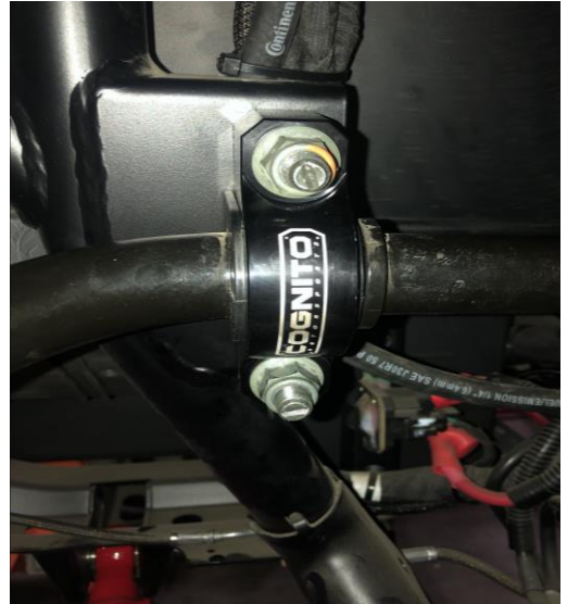
Figure 5: Billet Mount Installed
