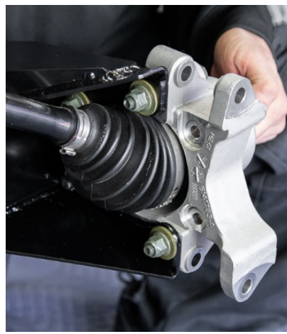
Figure 18B: Axle Installed
