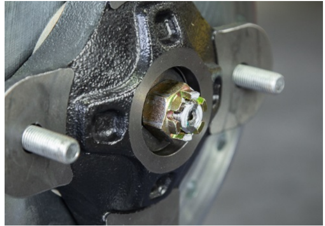
Figure 21B: Hub Nut Installed
