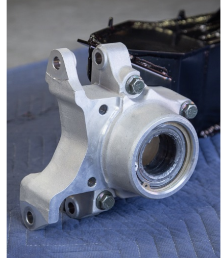
Figure 15C: Bearing Carrier Installed
