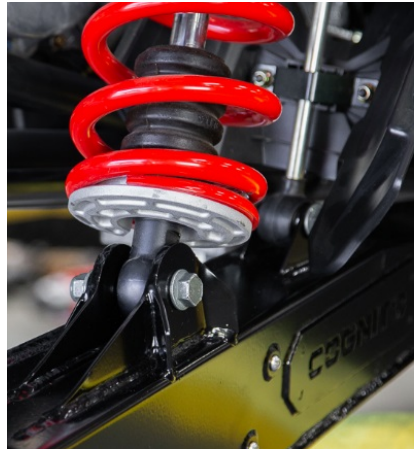
Figure 17B: Shock Installed
