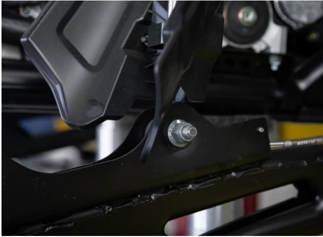
Figure 5A: Rear Sway Bar End Link Removal
