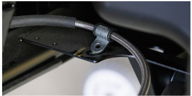
Figure 1B: Mounting Bolt Removed
