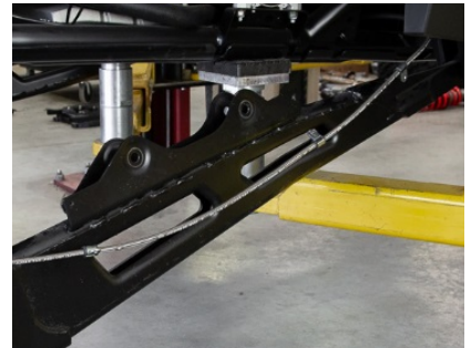
Figure 7C: Brake Line Removed
