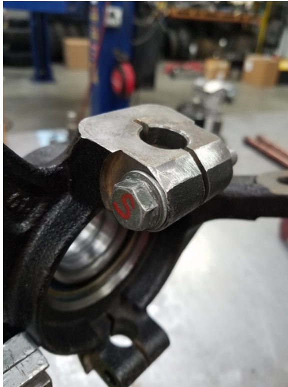
Figure 5: Grinding done on inboard side of top, material removed right up to the flange of the bolt and nut.
