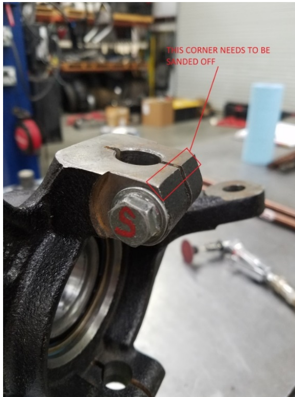
Figure 3: more detail shown of the area that needs to be removed, which must be done in both locations shown in Figure 1.
