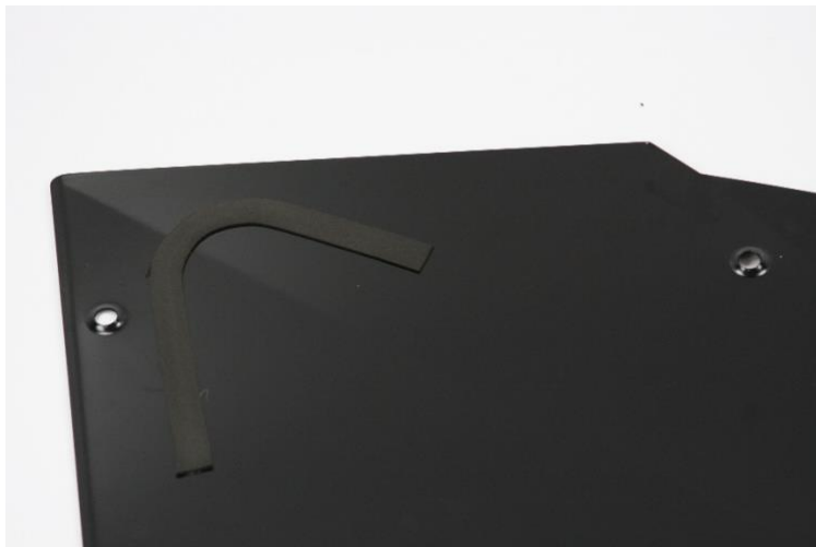
Figure 7: Foam around path of 1/2" tube on rear driver door.
