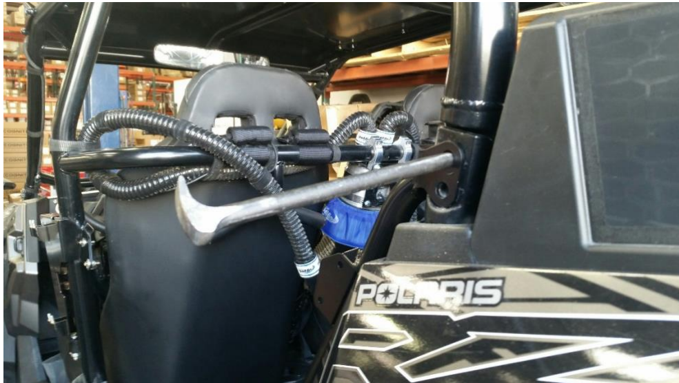
Figure 1: Use a ladyfoot pry bar to help line up the holes between the bracket and the frame cage. Then insert frame bolt and tighten to prevent the cage from springing back. Remove ladyfoot pry bar and insert upper bolt.
