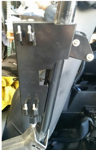
Figure 3: Center door adapter plate attached to car. Driver side shown.
