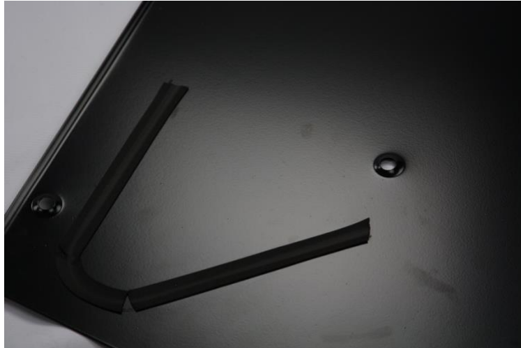
Figure 5: Foam around path of 1/2" tube on front driver door.
