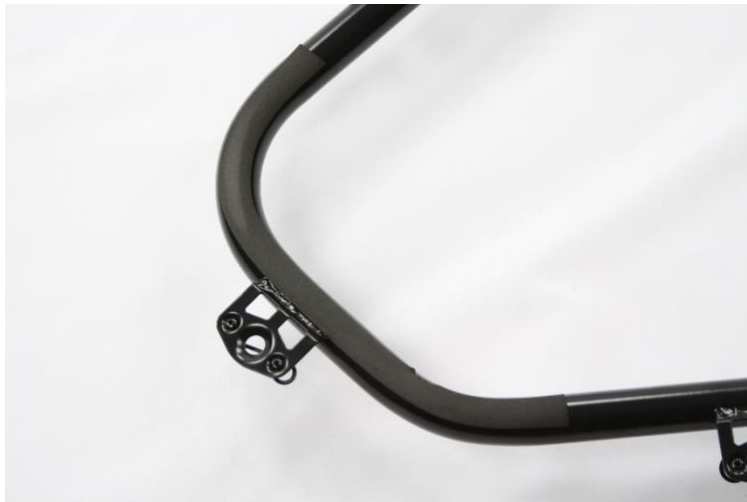
Figure 6: Foam applied to front lower corner of front driver side door tube.
