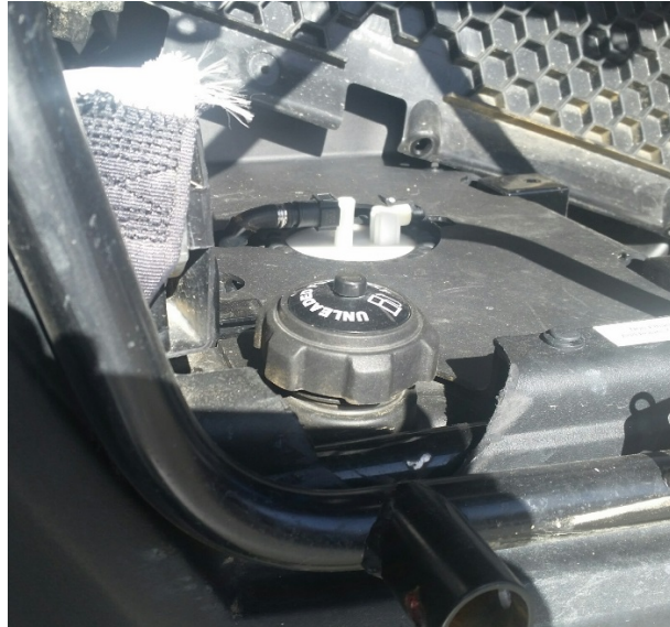
Figure 1: Trimming the plastic around the gas cap as pictured will allow for the door tube to sit closer.
