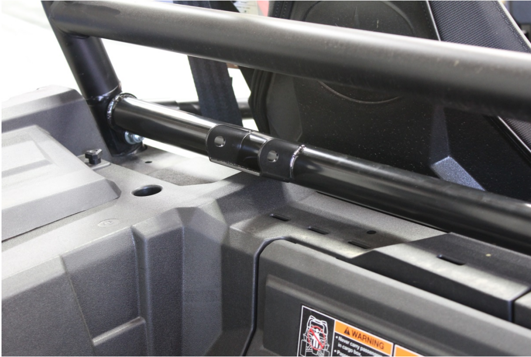
Figure 2: fit the universal mount bar in place, don't tighten yet, need to determine the combination of spacers that need to be used.
