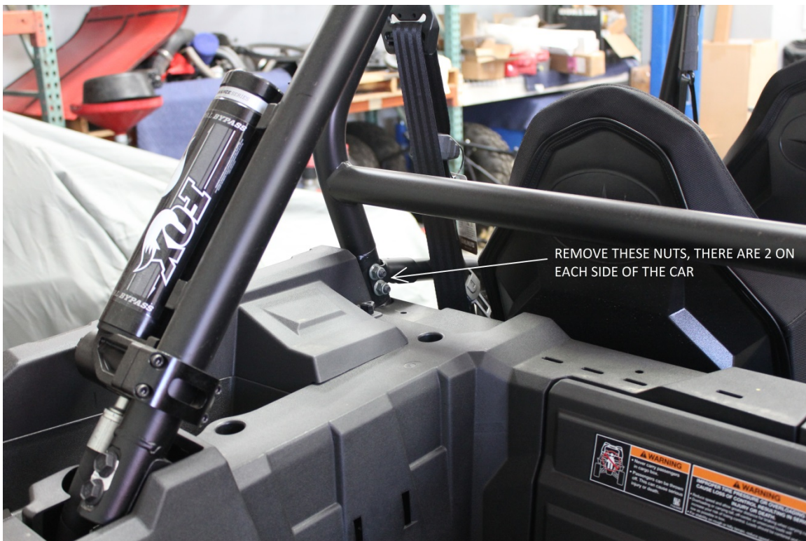
Figure 1: remove nuts, 2 on each side of car
