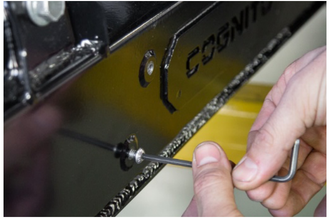
Figure 1B: Bolt Removal
