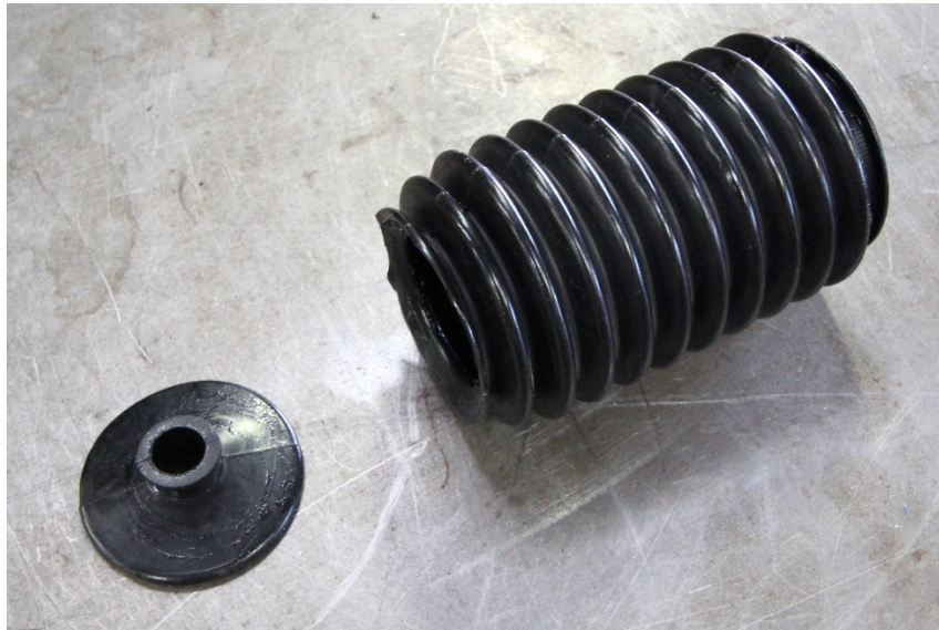
Figure 3: trim the small end off the dust boots, so it can be attached to the clevis groove.
