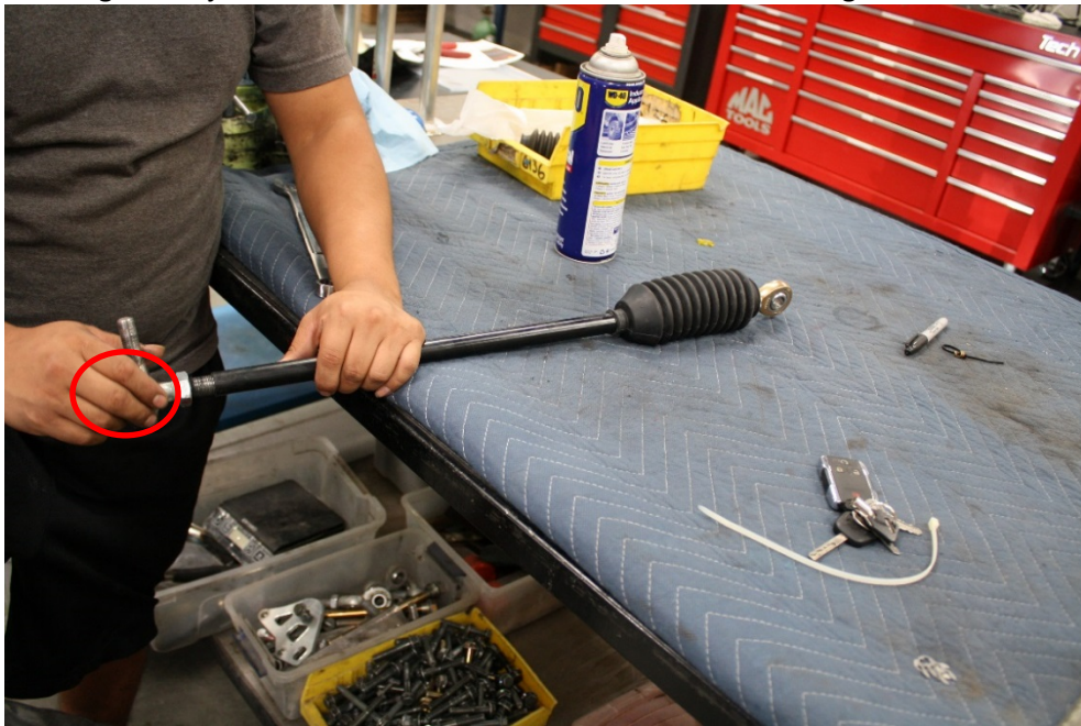
Figure 1A: Remove this tie rod end and install dust boot from here.
