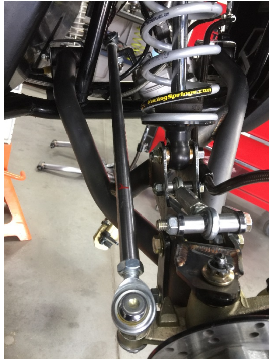
Figure 2: The position of the tie rod should be as pictured.
