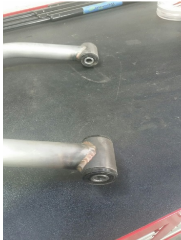
Figure 2: Picture showing bushings and crush sleeve properly pressed into pivot tube of the control arm.
