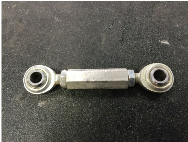
Figure 6: Camber adjuster rod assembled. Right and left handed heims, and jam nuts, are utilized so turn accordingly to assemble.
