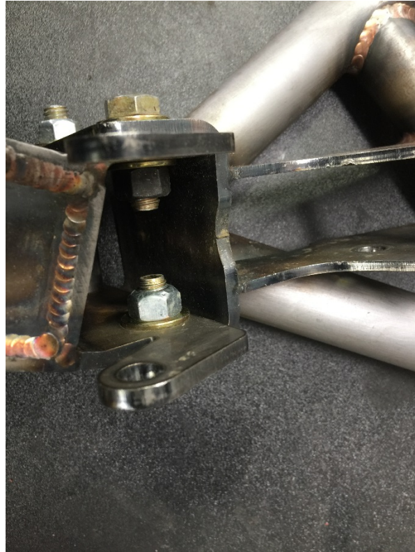
Figure 5: The 3/8"-16 x 1" bolts running through the camber adjustable slot holes.
