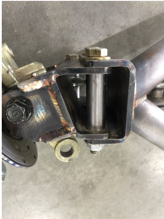
Figure 4: The crush sleeve goes on the bottom side of the control arm.
