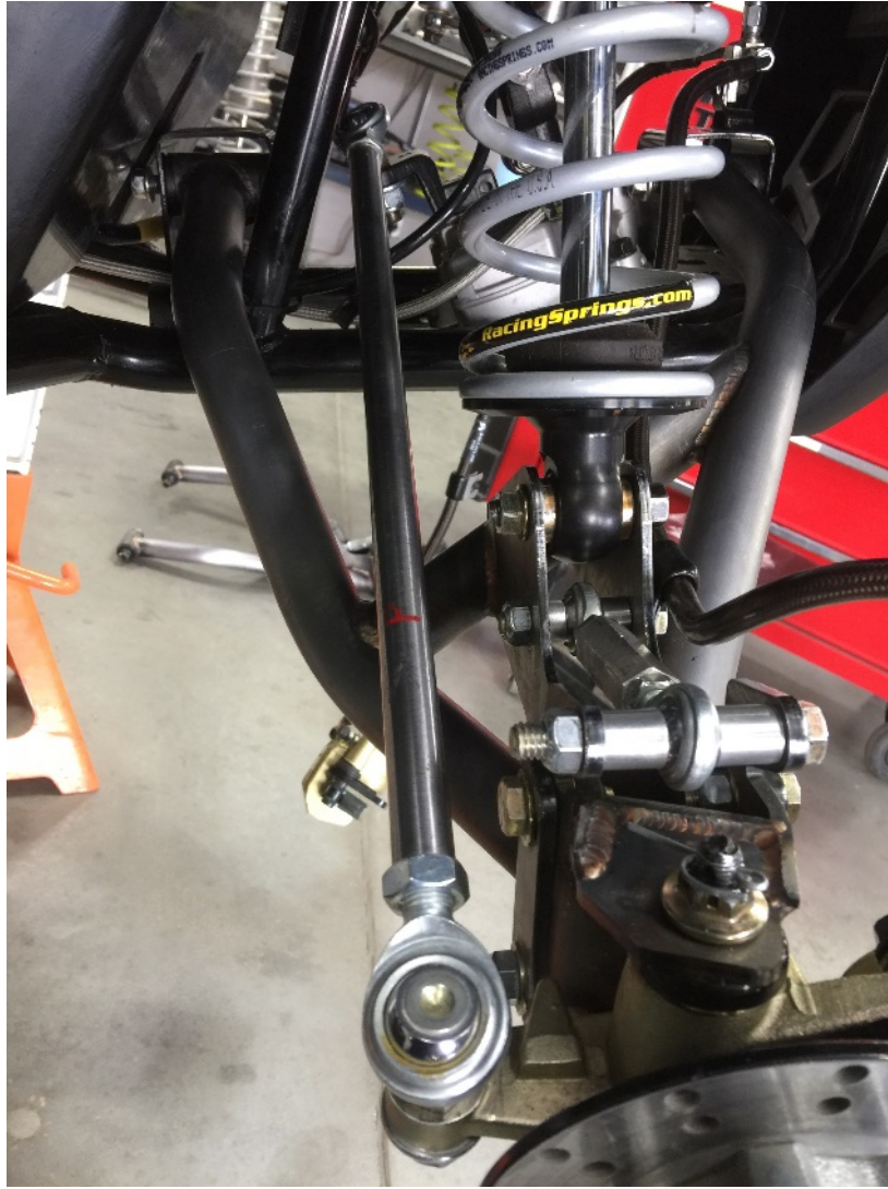
Figure 8: The position of the tie rod should be as pictured if using the Cognito Tie Rod kit.
