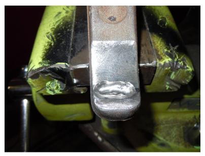
Figure 19: Use a carbide grinding bit to connect the 2 countersink spots in order to create an oval shaped pocket as shown. Now ready to install.
