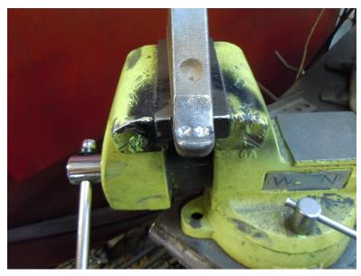
Figure 18: using a drill motor and 1/2" drill bit, drill only 1/8" deep from the tip so create 2 counter sink spots.
