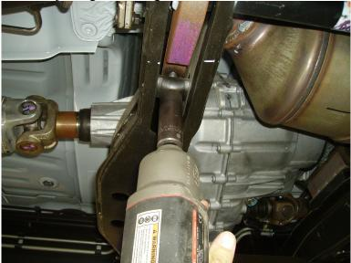
Figure 1: remove torsion bar adjusting bolt
