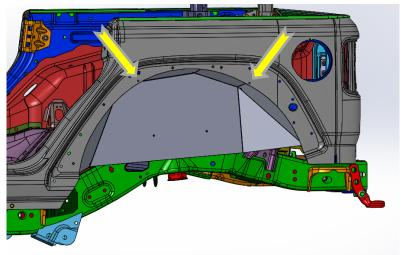
4. Using a torx 30, install two 6mm bolts in the locations shown below. Make sure to install the provided spacer behind the inner fender in these two locations.
