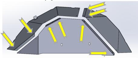
2. Attach two 6mm clip nuts to the locations shown below.
