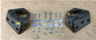
4. Using a 9/16" socket and wrench, a ¾" socket and wrench, and hardware from hardware kit #186, attach the frame mounts to the frame of the truck. Use 1 bolt, 2 flat washers, 1 lock washer, and 1 nut per hole. Do not fully tighten.
