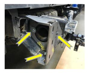
5. Using a hoist or a few friends, attach bumper to frame mounts using hardware kit #58 and the two provided weld-nut tabs. Start all bolts before aligning bumper. Open the tailgate slowly to ensure clearance below tailgate and bumper. Tighten all bolts with 3/4" and 9/16" sockets and wrenches. Torque all bolts to spec on page 1.
