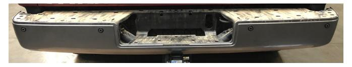
7. Use a T45 Torx Bit to remove the 6 bolts attaching the bumper to the frame. There are 4 on the top, and 2 underneath the bumper.
