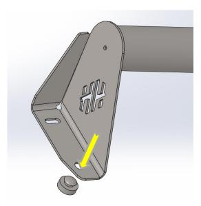
2. Using a Torx 45, mount the Speaker Pod Mount on rollcage with the two provided 3/8" bolts in the locations shown below.  $\setminus$
