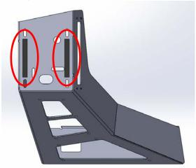
3. Using scissors, cut four 13.75" (350mm) length foam strips and apply two of them to the bottom of each upright (See Pic)
