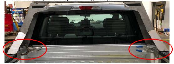
3. Using hardware from hardware kit #159, the nylon clamp block, and the nylon clamp spacer, secure the uprights to the side of the bed rail. Insert two Torx 40 bolts and two flat washers through the two slots on the side of the upright. Insert one ½" hex bolt and one flat washer into the nut on the bottom of the upright. (See Pic) Do this for both sides. Use a Torx 40 bit and a ¾" socket or wrench to tighten the bolts
