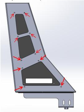
5. Locate the Left Bar Bracket and the Right Bar Bracket. Install the brackets on the ends of your 50" light bar. (See Pic)
