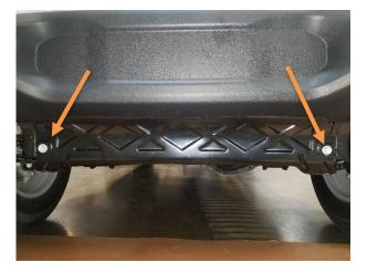
3. There is two nuts on the outside of the frame and the inside of the frame for a total of 8. Remove these with the 18mm socket.
