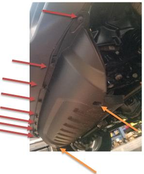
2. Remove the two bolts from the backing plate with the 15mm socket then remove the plate.
