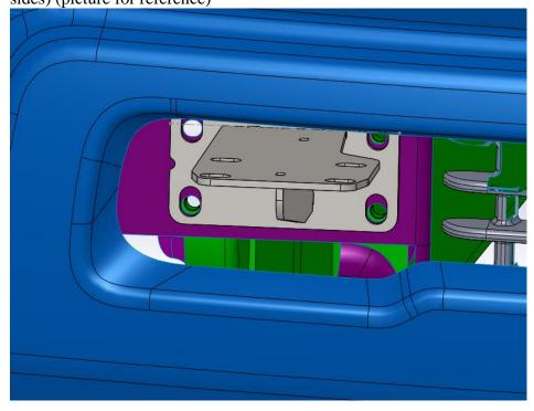
3. Lay down carpet or cardboard in front of truck. Lay Bull Bar as shown. Use hardware kit #92 to attach bull bar to frame mounts. Use one 3/8"-16 bolt, one 3/8" lock washer, and one 3/8" flat washer per hole. Install all bolts. Using a 9/16" socket with 3" extension, tighten all bolts. Use torque values on page one.
