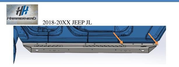
6. Install three torx 40, 8mm bolts and washers into the underside of the body.
