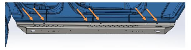
5. Install two torx 20, 6mm bolts and black washers where you removed the two factory fender bolts.
