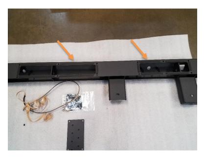
2. Using the twelve 1/4" carriage bolts, washers and nuts install the step plates as shown. You will use the 7/16" wrench or socket for this step. Make sure the step perforations are sticking up for grip.
