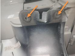
7. Lift the hood and remove the indicated plastic Christmas tree. Once it is removed you will be able to lift up on the center cowl and slide the side cowl in place.
