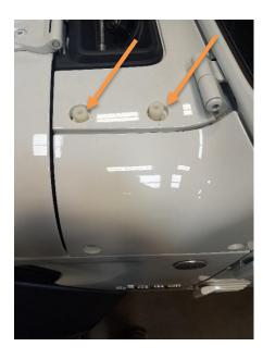
2. Install the short spacers on the bottom two holes as shown.
