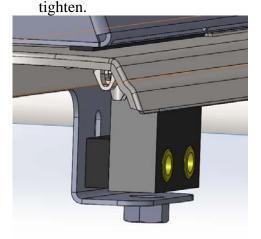
Place one flat washer on one Torx 40 bolt and insert through slot, nylon spacer, and into nylon clamp block.
