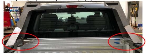
3. Using hardware from hardware kit #159, the nylon clamp block, and the nylon clamp spacer, secure the uprights to the side of the bed rail. Insert two Torx 40 bolts and two flat washers through the two slots on the side of the upright. Insert one ½" hex bolt and one flat washer into the nut on the bottom of the upright. (See Pic) Do this for both sides. Do not fully
