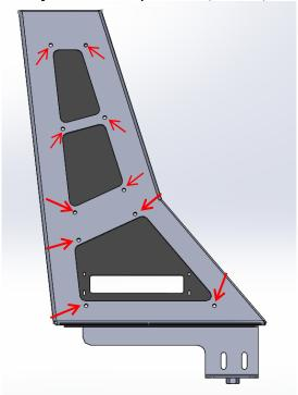
5. Locate the Left Bar Bracket and the Right Bar Bracket. Install the brackets on the ends of your 49.5" light bar. (See Pic)
