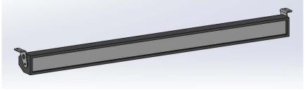
6. Once the brackets are installed on the light bar, install the light bar into the top cap weldment using hardware from hardware kit #158. Insert four carriage bolts through the top cap weldment and the brackets (see pic), and then secure it using the provided flat washers and nylock hex nuts. Use a ½" socket to tighten the nuts.
