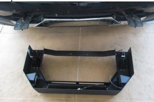
5. Have a friend help you align the Bull Bar. Push top of Bull Bar toward truck. Using a <sup>3</sup>/<sub>4</sub>" socket and wrench, tighten frame mount bolts at this time. Use torque values on page one. Verify top of Bull Bar is level with ground. The Bull Bar needs to be close to the truck to allow sensor functionality.
