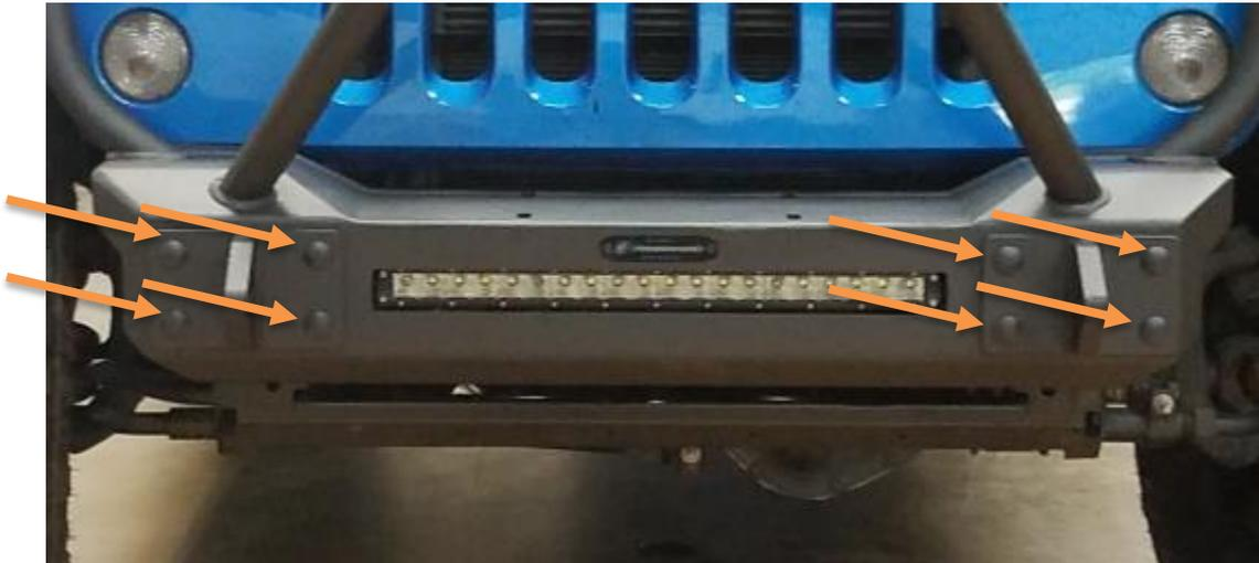
5. Align bumper and torque all bolts to spec
