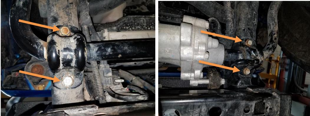
4. Place bumper on Jeep. Using 8 black 1/2" carriage head bolts install the bumper. Bolts go through the shackle mounts, then the bumper. Use the provided 1/2" nuts, washers, and lock washers to secure the bumper.
