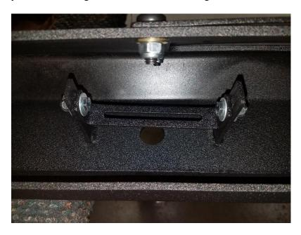
4. Bolt the rock rail to the jeep with the 2 body mount bolts you removed earlier as shown using the 18mm socket.
