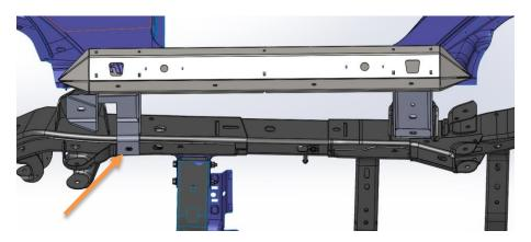
6. Install the provided 3.5in .5in bolt, nut, and washers from hardware kit #111 in the shown location. You will use the ¾" socket and ¾" wrench. Bolt will go all the way through the frame.
