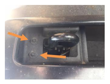
2. Using an 18mm socket, remove the 2 bolts. Be careful not to lose the backing plate located behind the bumper.
