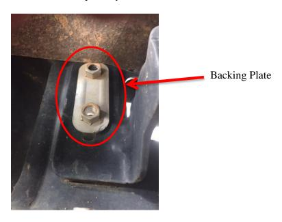
3. Using the OE hardware, install the frame mount around the tow hooks and tighten both bolts.
