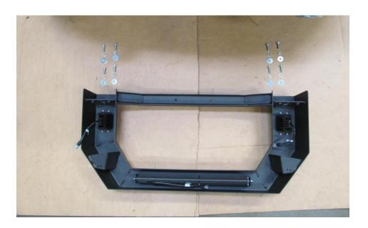
6. Have a friend help you align the Bull Bar. Push top of Bull Bar toward truck. Use torque values on page one. Verify top of Bull Bar is level with ground.
