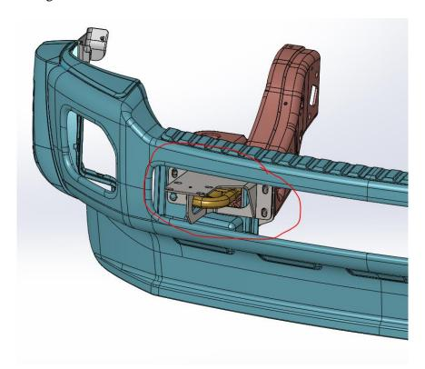
4. The brace bracket will mount from the side of the frame horn to the back of the bull bar mount. (See Pic below)
