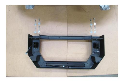
6. Have a friend help you align the Bull Bar. Push top of Bull Bar toward truck. Using a 5/8" socket and wrench, tighten the frame mount bolts at this time. Use torque values on page one. Verify top of Bull Bar is level with ground.
