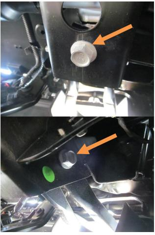
2. Using an 18mm socket and wrench, remove the tow hook bolts and the tow hooks. Set the hooks and OE bolts to the side, you will not use them again.
