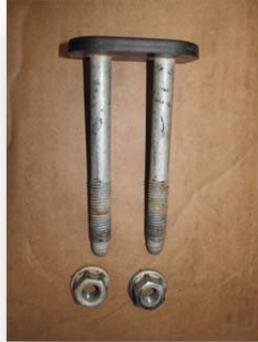
4. Using 18mm socket and wrench remove the bolts attaching the tow hook to the frame. Remove tow hook and set aside. (both sides).
