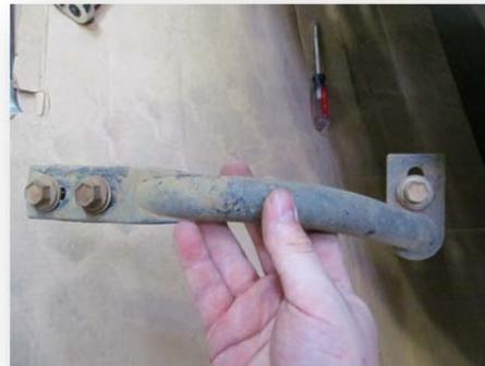
3. Using a 21mm socket remove two nuts from the bolt strip attaching the bumper to the frame of vehicle. (both sides)
