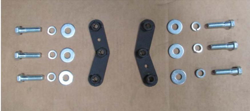
5. Using a hoist or a few friends, attach bumper to frame mounts using weldnut tabs and hardware kit #58. Insert bolts front the center of the bumper. Start all bolts before aligning bumper. Align bumper a minimum of  $\frac{1}{4}$ " below headlights. When truck flexes off-road, this distance allows your bumper and body to have clearance. Tighten bolts with  $\frac{3}{4}$ " socket. Tighten all hardware.
