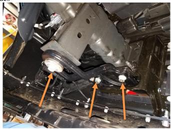
2. Remove the three 18mm nuts shown. Once done you can remove the tow hook bracket. Do this for both sides
