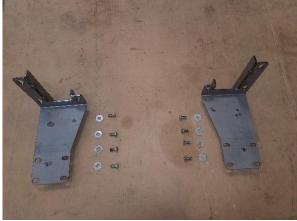
2. Install frame mount through bumper's tow hook cutouts. It is easiest to come from the back and rotate them in as you slide them forward. Use the three OE 18mm nuts to bolt on the frame mounts.
