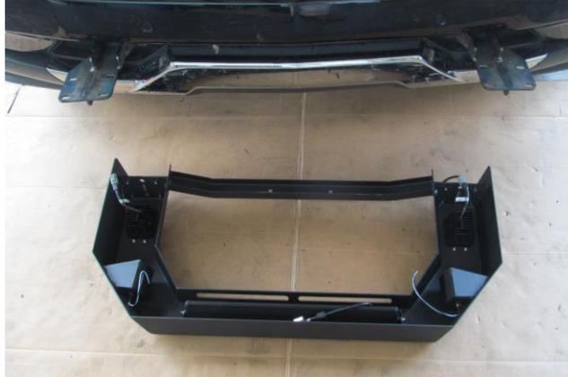
5. Have a friend help you align the Bull Bar. Push top of Bull Bar toward truck. Using a 3/4" socket and wrench, tighten frame mount bolts at this time. Use torque values on page one. Verify top of Bull Bar is level with ground. The Bull Bar needs to be close to the truck to allow sensor functionality.
