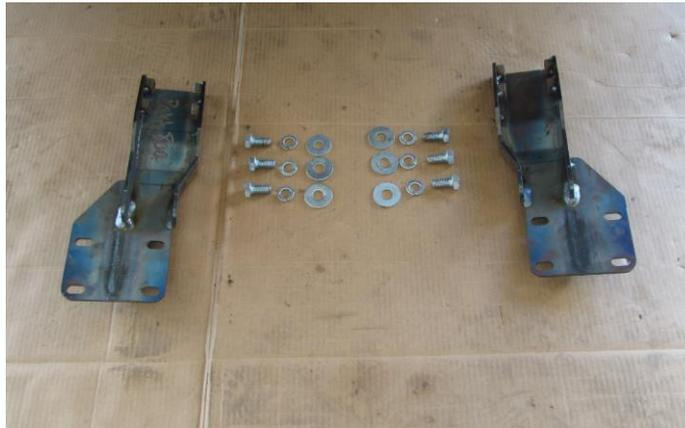
2. Install frame mount through bumper's tow hook cutouts. Use one 1/2"-13 bolt, one 1/2" lock washer and one 1/2" flat washer per hole. Hand tighten bolts.
