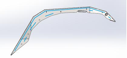
2. Place flare on the fender. The OE fender brace goes through the opening on the inside of the flare.
