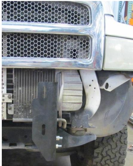
FIGURE 7: FRONT VIEW OF DRIVER SIDE FRAME MOUNT
