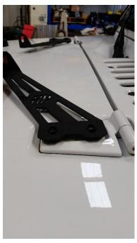
3. Using a Torx 40 socket place provided bolts 75% of the way in hood latch
