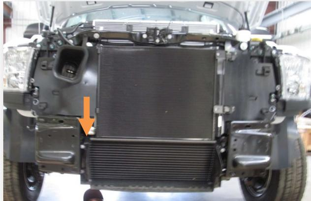
12. Remove bolt strip on Passenger side. (Bumper bracket will fall off once bolt strip is removed. Be mindful of any sharp edges on bracket)
