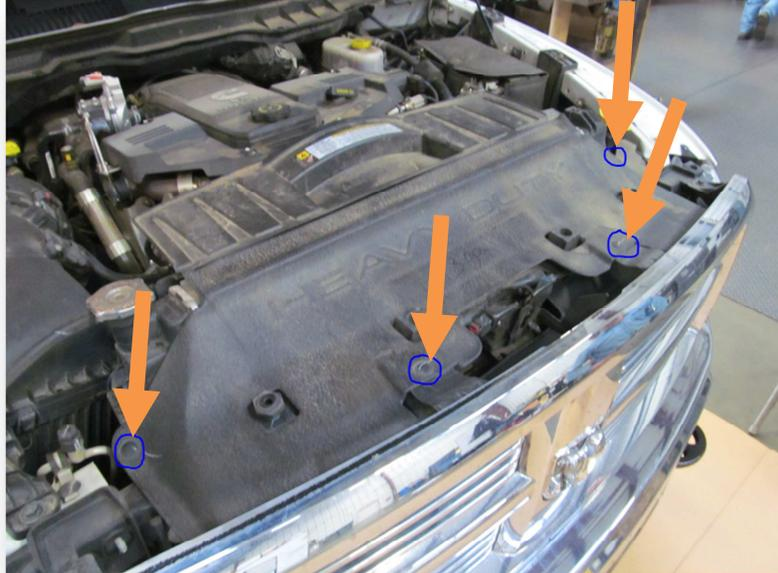
2. (Diesel only) Using a 10mm socket remove the grill by taking out four screws on top of grill. Pull gently on bottom of grill after screws are removed to release plastic tabs. Remove grill and set aside.
