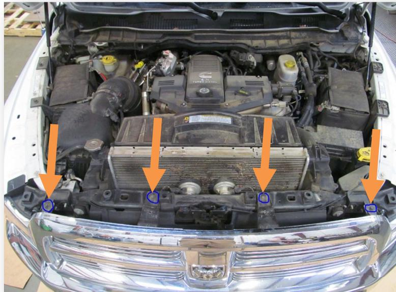
3. (Diesel only) Using a 13mm socket, remove two bolts holding top of intercooler.
