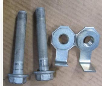
7. (On 4500's and 5500's) remove tow hooks from both sides and set aside.
