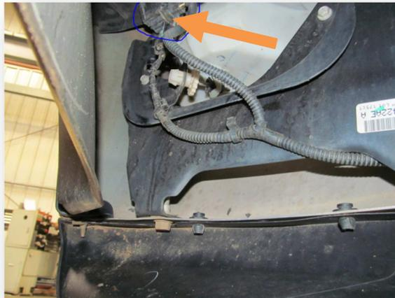
5. (Gas and Diesel) Using 18mm socket, remove two nuts that hold on the bolt strip (Be mindful of any sharp edges on bracket.) On diesel, carefully move one side of intercooler to ease in removal of bolt strip. (both sides) Carefully remove OEM bumper and set aside. Bolt strip will be reused to mount Hammerhead bumper.
