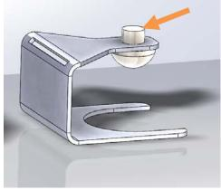
3. Slide sensor clip over grommet and ensure rubber bumper touches the back of the sensor. This clip will retain the sensor in the grommet.
