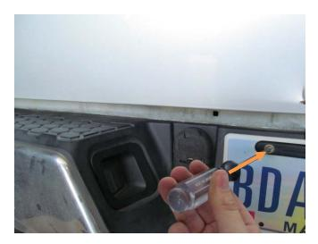
4. Behind the license plate there are either two bolts or two nuts depending on year model. Use 15mm socket to remove both of them.
