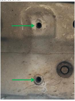
2. Using M8 bolts from hardware kit #75, Thread bolts in and out of inserts to verify threads are clean of debris.
