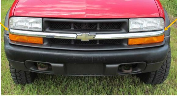
2. Now you will remove the bumper outer bolts. They are located in front of the tires. Using a 15mm socket, remove the bolts, attaching the side braces to the bumper. Then remove the two bolts attaching the side braces to the frame. Remove brace and set aside.
