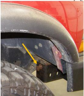
3. Install HH bumper on truck and use OEM bolts to attach top of bumper (see pic) to OEM mounts. Do not fully tighten.
