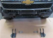
3. Attach Hammerhead frame mounts to OEM frame with OEM bolt strips. Push mounts to top of slots and tighten.
