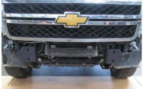
4. In this step you will use hardware from kit # 1. Install and align Hammerhead bumper using six ½" -13 x 2" bolts, 12 ½" flat washers, six ½" lock washers and six ½"-13 nuts. Use this hardware to attach bumper to HH frame mounts.
