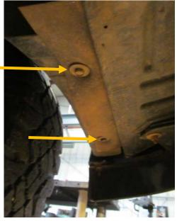
4. Using 15mm socket, remove three bolts attaching side bumper brace to frame. Set brace aside. (both sides)
