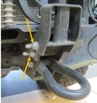
10. Using 18mm socket and wrench, remove two bolts attaching OEM tow hook to frame. Set tow hook aside. (both sides)
