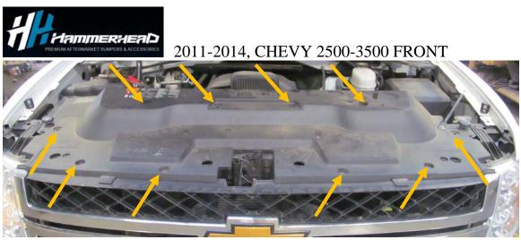
6. Using 10mm socket, remove four screws attaching top of grill to truck. Screws will be reused.
