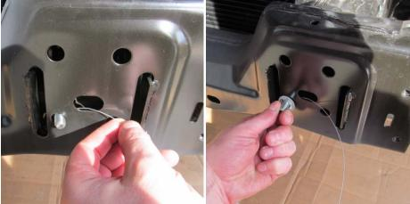
(C) Thread 10mm-1.25mm nut on bolt. While holding nut, slowly pull wire to remove it from bolt and engage push nut fully on threads. NOTE: Bolt may try to back out of nut while pulling wire.
