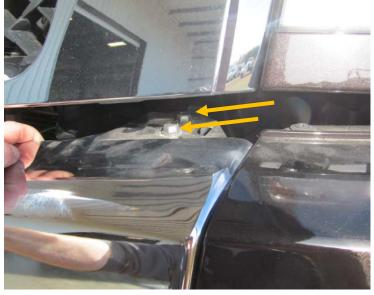
7. Using a 17mm socket, remove two bolts holding tow hooks to frame. Remove tow hook and set aside. (both sides)
