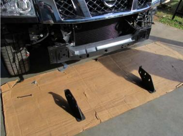
2. In this step you will use hardware from kit #13. Using 10mm-1.25mm x 25mm bolts (qty-4), lock washers (qty-4) and flat washers (qty-4), install frame mounts as shown. The bolts will thread in bosses in the frame. Do not fully tighten. (both sides)
