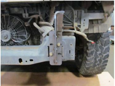
3. In this step you will use hardware from kit #1. Install bumper on frame mounts. Each mount will use ½"-13x2" bolts (qty-3), ½" flat washers (qty-6), ½" lock washers (qty-3), and ½"-13 nuts (qty-3). Align bumper and tighten all hardware.
