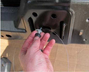
(D) Remove nut.(E) Repeat for the seven remaining bolts.
