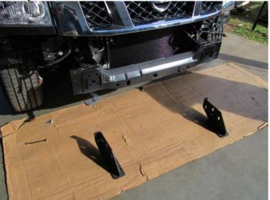
4. Install frame mounts on bolts. Use 10mm flat washers, 10mm lock washers and nuts to secure frame mounts. Hand tighten nuts.
