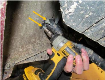
3. Using a 17mm socket, remove two bolts holding the bumper brackets to the frame. (both sides)
