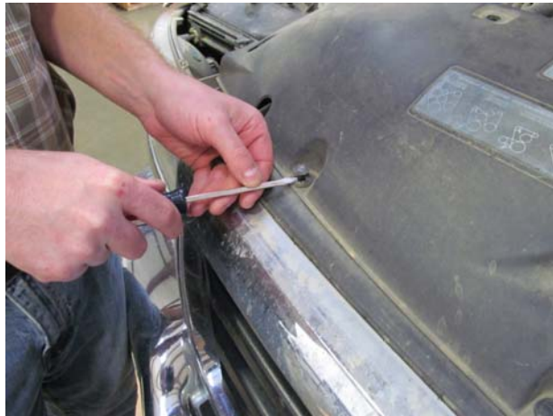
FIGURE 1. REMOVAL OF CHRISTMAS TREE CLIPS
