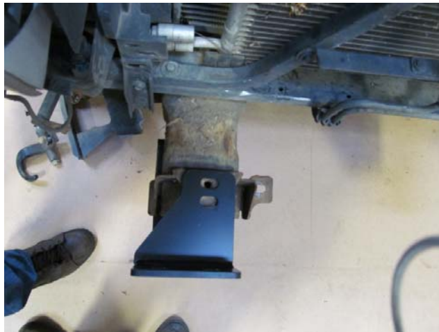
FIGURE 15: TOP VIEW OF FRAME MOUNT
