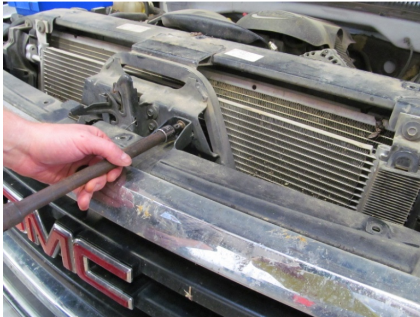
FIGURE 2. REMOVAL OF TOP GRILL BOLT
