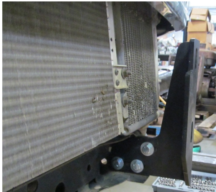
FIGURE 9: INSIDE VIEW OF FRAME MOUNTS
