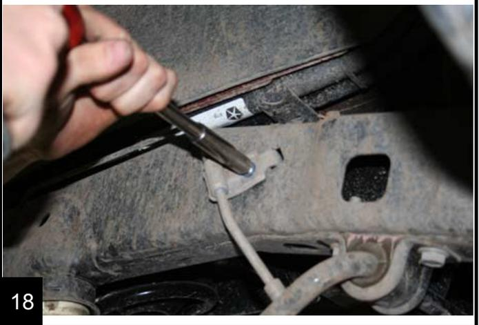
Carefully lower the axle enough to remove the spring. Be sure to watch the ABS, brake lines and breather tubes for overextension. Remove the old spring.
