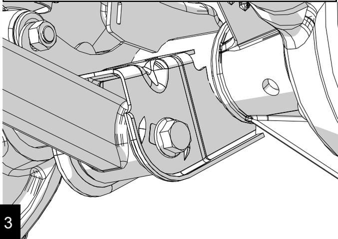
Remove the shocks at the axle with an 18mm wrench and socket.
