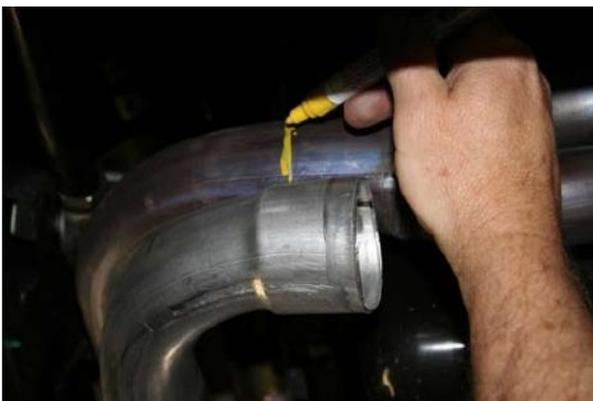
Cut the exhaust at your mark near the front corner of the oil pan, and remove the rest of the exhaust system including the catalytic converter, muffler and tailpipe. Be very careful to avoid damage to the oxygen sensor and wiring. Make the second cut on the exhaust where you made the mark a few inches in front of the catalytic converter and reinstall the exhaust at step 26. When you have the new muffler and tailpipe built
