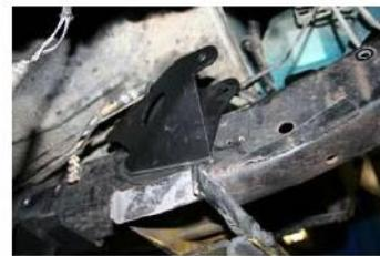
22. Weld the bracket to the frame and paint the weld area to prevent rust.
