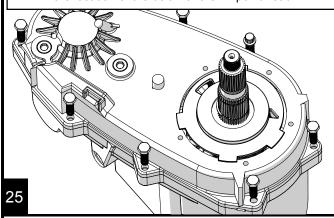
Install a new snap ring (1), followed by the speedometer gear (2), install the final snap ring (3) to retain the gear.
