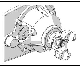
Install the rubber seal washer on front output, install yoke. Apply red thread locking compound to nut and torque to 90-130 ft-lbs
