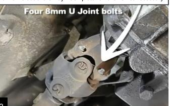
Remove the front output yoke.
