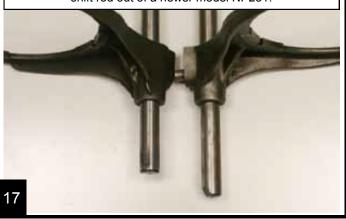
Install the new main shaft, chain and front output.
