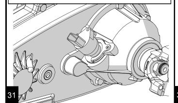
Torque the sensor bolt 8-12 ft-lbs. XJ applications, install the vacuum switch into the tail housing. Torque to 15-25 ft-lbs.
