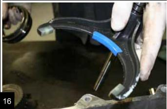
Verify the length of the mode fork shift rod is 9.38". Typically 1988 and 1989 YJs and XJs have a mode fork shift rod that is 10.2". Simply cut the shift rod as shown, or purchase a shift rod out of a newer model NP231.
