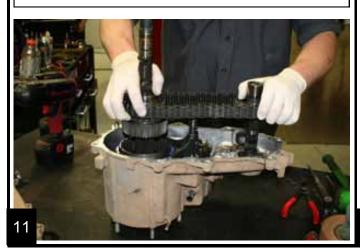
Remove the synchro hub snap ring and remove the hub and drive sprocket from the main shaft. Note the orientation of the hub and drive sprocket.
