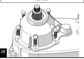
Apply a small amount of silicone to seal the spline and yoke interface under the yoke nut. Apply red thread locking compound to the yoke nut and torque to 90-130 ft-lbs.
