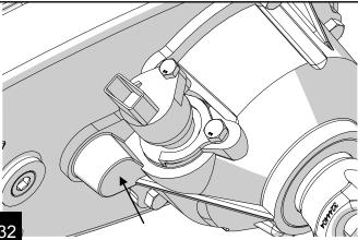
Fill transfer case with 2.2 pints (1.0L) of ATF+4 and reinstall into vehicle if transfer case was removed.
