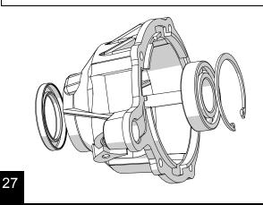
Apply a maximum 3/16" bead of gasket maker to the new tail housing, install and torque bolts in a crisscross pattern to 15-20 ft-lbs.
