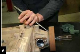
Remove the rear output shaft seal.
