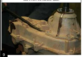
Split the case by removing the 8 case half bolts. Note the location of the 10 mm 12 point bolt.
