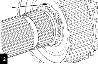
If your transfer case comes from a 1996 or older vehicle, it may be necessary to remove the needle bearings in the drive sprocket. Drive them out using a large socket and hammer.
