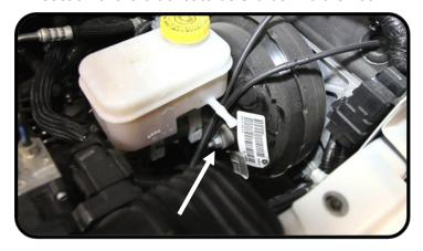
Position the pump/bracket assembly such that the hole in the bracket lines up with the threaded fender hole as shown, and slide the slotted portion of the bracket behind the previously loosened nut and over the stud.
