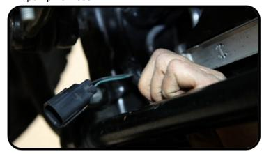
16. Strip 3/8" of the insulation from the two wires protruding from the factory connector and attach the supplied green and black wires to the factory connector using the supplied heat-shrink butt connectors.
