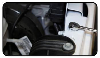
5. Loosen the 13mm nut on the driver's side brake booster stud far enough to enable the slotted section of the bracket to be slid behind the nut.
